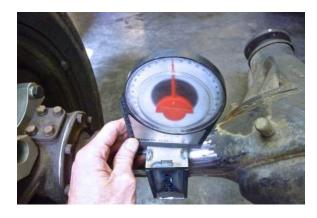
Insure that the front axle assembly is level using an angle gauge. If it is not level; level it by placing it on jack stands or something similar.
