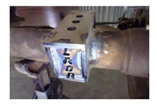
Place the rear axle assembly on (2) jack stands and remove both rear wheel assemblies using a 19 mm socket. This will allow better access to the spring pads for welding.
