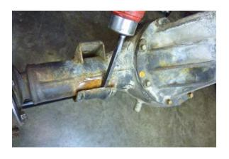
Work the U-bolt guide plate away from the axle housing using a hammer and cold chisel.
