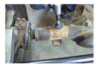
Remove any rust and paint in preparation for welding by using an angel grinder with "Flap Disc" or equivalent.
