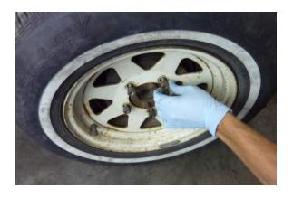
Replace both wheel assemblies and progressively tighten the lug nuts in a criss-cross pattern until 36.5 to 57.5 ft. lbs. is reached.
