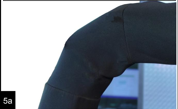
Remove the driver and passenger foam pads from the sports bar and make a mark that is 4 1/4" from the back using the mold seam as a guild. Using a utility knife cut the foam pad.
