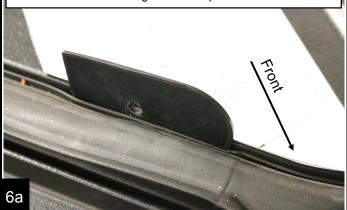
Center templates on outside rib as shown. Hold templates with a small length of painters tape.
