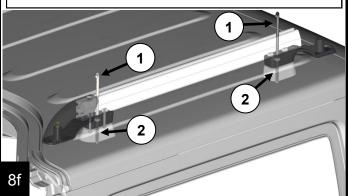
With the #393 torx tool centering the main rail access holes over the #220 M8 mounting bolts tighten the #729 M6 shoulder screw (1) and #225 M6 flat socket head (2) installed in step 8d & 8e. Repeat steps 8d to 8g for the other side.
