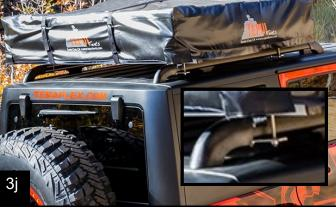
Many aftermarket crossbars/ load bars will fit around the main rail, allowing various carriers to be mounted Shown is a Thule AreroBlade with the 450R Rapid Crossroad Foot Pack. Thule SquareBars can be mounted with the 450 Crossroad Foot.
