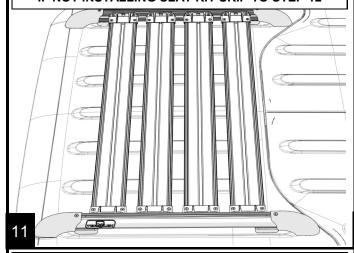
Press on one of the #772310 brackets (1) from the previous step on to a #772300 slat (4). Slide two #651390 t-nuts (3) into each of the two outer tracks, then press another #772310 bracket (1) on the other end. Repeat for all 4 slats.
