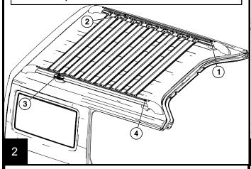
Follow the owners manual procedures for the rest of the OEM hardware. With a helper, pull the top straight up to free the bolts, then remove the top.
