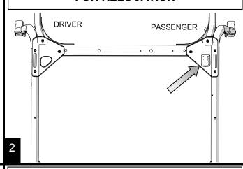
Using an 10mm wrench, remove the antenna mounting bolt and standoff spacer. Press in the lock tabs on the antenna and push the antenna out of the base plate.
