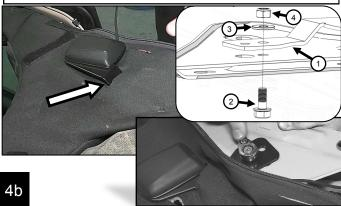
Apply thread lock to an OE M8 bolt (1) and install it through the base plate. **Do not tighten bolt.** Rotate the satellite bracket until the second holes line up in the satellite bracket and the base plate and tighten antenna bracket bolt to 14 ft-lbs (19 Nm).
