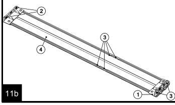
Slide a slat assembly from the previous step into the main rails. Be sure to line up the #651390 t-nut (1) to the upper slot. The tabs (2) on the #772310 bracket will line up with the lower slot. Slide slat forward and repeat for each slat.
