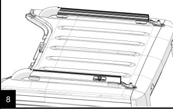
Ensure that the rail t-nuts (1) are loose. Install the passenger side rail by starting at the rear and sliding the rail forward as the T-nuts slide in the lower track. Stop sliding it forward when the front rail through hole is centered on the now cap-
