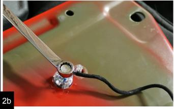
Using a 10mm socket, loosen the two screws on the passenger side of the speaker pod, gently pull down so the antenna connector can be removed. After the connector is removed, tighten the two screws to 90 in-lbs (10 Nm).
