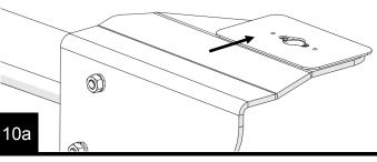
If using shims in the front, trim the back edge of the front shims with an X-ACTO Knife so it does not overhang.
