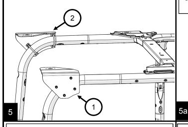
Unzip the covers from the driver and passenger side sport bar at the rear of the Jeep. Seat belt does not need to be removed.
