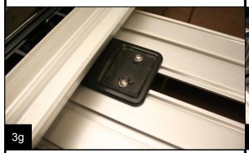
Below is a Quick Fist mount installed with a M6 x1.0 x 22mm long bolt with a washer under the head to avoid bottoming out.
