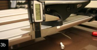
Internal view of the Thule Xadapt10 being installed in the sonic box with a M6 x 1.0 x 30mm long screw.
