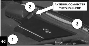
Install the #772230 bracket (1) to the OEM base plate using the OEM M8 hardware (2). (APPLY THREAD LOCK TO BOLTS) Use a 13mm to tighten bolt (3) under the antenna bracket to 14 ft-lbs (19 Nm). Leave the other three M8 bolts (2) loose so the support bracket can be shifted easily. Cover omitted on drawings for clarity.
