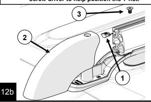
Thread the #225 M6 bolt (1) with a #459 washer (2) though the rear most hole in the hard top and into the cap (3), see section view below.
