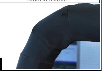
Remove the driver and passenger foam pads from the sports bar and make a mark that is 4 1/4" from the back using the mold seam as a guild. Using a utility knife cut the foam pad.
