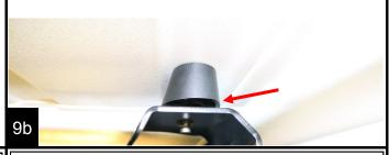
NOTE: If mounting bolt (1) contacts the OEM lower bracket (2) the hard top will need to be removed to modify the OEM bracket. If there is no contact with bolt skip forward to step 9f.
