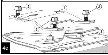
On the driver front side remove the three rear most base plate bolts. Slip the tabs of the #772231 Front Drivers Side Bracket (1) through the slit in the cover, as shown in 4d, then repeat step 4e for the support bracket. (APPLY THREAD LOCK TO BOLTS) Leave the bracket loose so it can be shifted easily.
