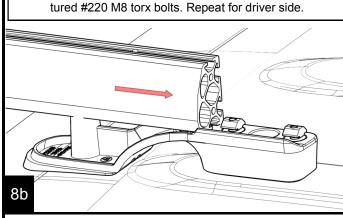
On the driver front mount(2) insert a #2035 Oring (7) into the cavity. Next insert a M6 t-nut (3) into the top slot of the main rail. Position the #772151 cap(1) onto the rear foot and install on a #729 M6 Flat Head Bolt(4) into the top hole of the cap and into the T-nut.
