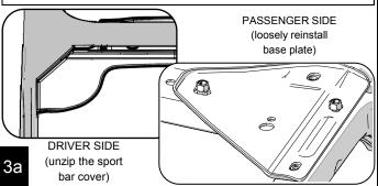
Align the outside edge of the front passenger template (722194) to the edge of the zipper tape. The other edges will align with the base plate under the cover. Slit the cover in the 4 locations marked on the template.
