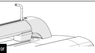
Slide a 13mm open end wrench under the front of the hard top to lightly snug up the (1) OE M8 inner front bolt for both the driver and passenger front mounting brackets.
