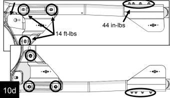
Install two of the #729 M6 flat screws (2) and two of the #651390 M6 t-nuts (3) loosely in the locations shown on all eight of the #772310 mounting brackets (1).
