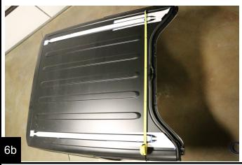
Adjust templates so they are both centered on the rib and measure 43-15/16" [111.6cm] from centerline to centerline. Measure across hard top at both the front and the rear 11/32" [8.7mm] marked holes on the template. When the measurement is correct secure template with painters tape.
