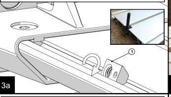
to mount an accessory, measure the thickness of the mounting foot and add 7.5 mm for thread engagement in the t-nut.
