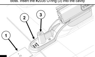
On the passenger side insert a M6 t-nut (1) into the top slot of the main rail. Position the #772151 cap (2) onto the rear foot and install on a #729 M6 flat socket screw (3) into the top hole of the cap and into the T-nut. TIP: Use a small flat bladed screw driver to help position the T-nut.
