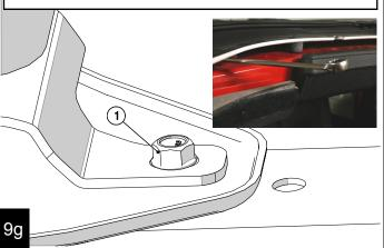
Snug down the 2 rear bracket clamps for both the passenger and driver rear brackets to keep the bracket from shifting. Remove the four #220 M8 torx bolts installed in
