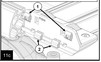
Position the slats along the main rail as desired, keeping the slat perpendicular to the rails. When in position, slide a t-nut (3) under the bracket (1) and thread a M6 flat cap screw (2) into the nut. Repeat for all lower holes. Tighten all upper/ lower M6 flat cap screws (2) to 105 in-lbs [12 Nm].
