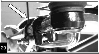
Perform a final check of the suspension components and bolts.
