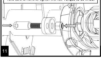
Insert the upper stud of the quick disconnect sway bar linkage into the factory sway bar. Place washer 477 and nylock nut 44 onto the stud.
