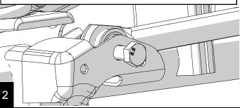
2011+ JK's have brake line retainers located under the spring perches. Use vise grips or a heel bar to spread the bracket enough to free the brake line. Use a 10mm to remove and discard the bracket.
