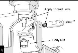
Torque the body mount to **80 ft-lb** and jam nut to **59 ft-lb**.
