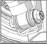
Install Front Swaybar Links in Place of Rear Links Install the replaced front swaybar links in place of the rear links. The ball joint stud end on top and with the mounting stud pointing towards the frame.
