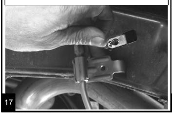
Fully remove the part brake cables from the hanger bracket and discard the bracket.
