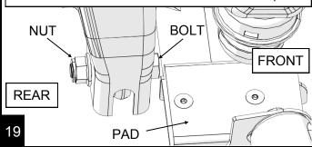
**IMPORTANT NOTE!** It is imperative at this time to cycle the swaybar and check for proper clearance between the swaybar and the brake line. Make the necessary bends in the brake line and bracket to clear the swaybar link as it goes through its range of travel.
