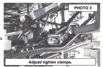
3. Install the new track bar into stock frame bracket using the stock hardware. Check to make sure the body is centered over the axle and install the lower end of the new track rod on the axle as shown in Photo 3. Torque fasteners to 125ft -lbs. It may be necessary to turn the steering wheel to align the track rod end with the axle. \*Note\* Make sure the jeep is sitting on the ground at ride height before tightening track bar bolts.
