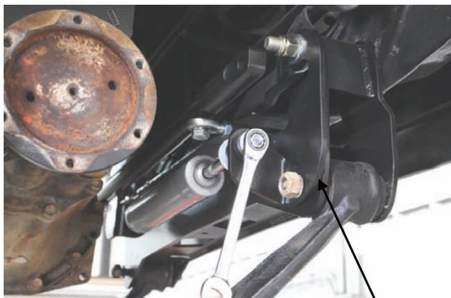
**Install the stab mounting bracket.**
