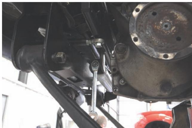
**Tighten the stabilizer mounting hardware.**
