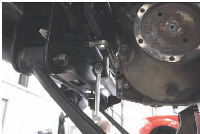
**Tighten the stabilizer mounting hardware.**
