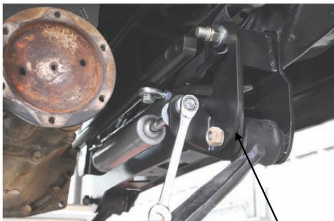
**Install the stab mounting bracket.**
