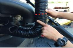
26. Pierce the Duct (N) centered between the two wire reinforcements using a razor blade to cut the duct to length. Cut all the way around. Try to cut the duct straight around the center as close as possible.
