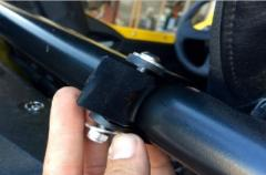
20. Use a 13mm wrench and 5mm Hex Key to install the Adapter (B) onto the bottom of the Particle Separator (A) with the supplied Screws (D), Washer (C) and Locknuts (E). Tighten these screws and locknuts.
