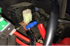
37. Insert the bottom cap and wire back into the Posi-Tap (V) making sure the strands go around the metal core. While holding the wire in place, screw the bottom cap back on until it is firmly tight. Double check both caps to make sure they are tight.
