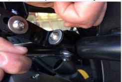
24. Install Hose Clamp #56 (O) onto the Duct (N). (Optional) For a cleaner appearance, take the end of the wire and tuck it inside the duct. Do this for both ends of the duct if desired.
