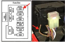
**33.** Unscrew the large top cap from the supplied Posi-Tap (V). Place the cap in between the wire.
