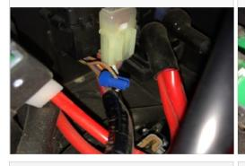
**36.** Unscrew the bottom cap on the Posi-Tap (V) and insert the Pig Tail through it.
