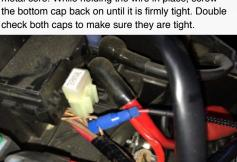
38. Find Fan Connector and connect it to the Particle Separator (A). Make sure not to cross the connectors. Power to power and ground (black) to ground (black). Note the color of the wires whenever connecting or disconnecting this connector. The connector should snap into each other with very little resistance. Do not try to force the connectors into each other.
