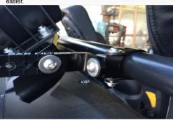
23. Once you are satisfied with the position, use a 4mm Hex Key and 10mm wrench to tighten the Screw (J), Washer (I), Locknut (K) at the Strap (H). Do this for both sides. Go over all the screws and locknuts again to make sure they are secure and that the Particle Separator (F) is firmly attached to the roll cage.
