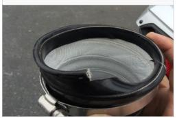
25. Insert one end of the Duct (N) and Hose Clamp (O) onto the Air Tube (M). Tighten the hose clamp at the air tube. Bring the other end towards the opening on the Particle Separator (A). Note the length on the duct you want to cut. We recommend cutting the duct an extra 3" longer so that the ends, along with any wire and strings, can be folded in for a cleaner look.
