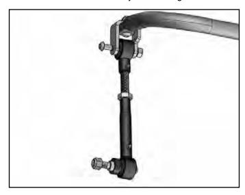
Slide the lower end of the Quicker Disconnect onto the tapered stainless steel post.
