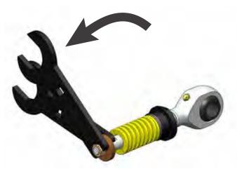
O Slide the spring off of the shaft.
