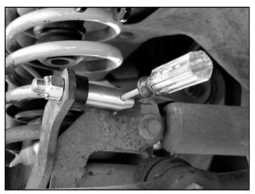
**HINT:** A small Philips head screwdriver or punch inserted into the Click Pin hole will enable you to prevent the tapered Stainless Steel Posts from rotating when tightening the Nylock nut.
