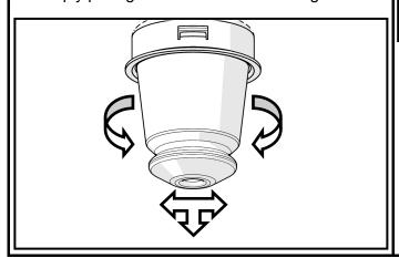
20. Install new bumpstop by twisting and pushing up. Note: If needed use a small amount of silicone lube spray, to help install the bumpstops.
