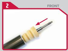
Orient and install bump stop on shock shaft as shown
