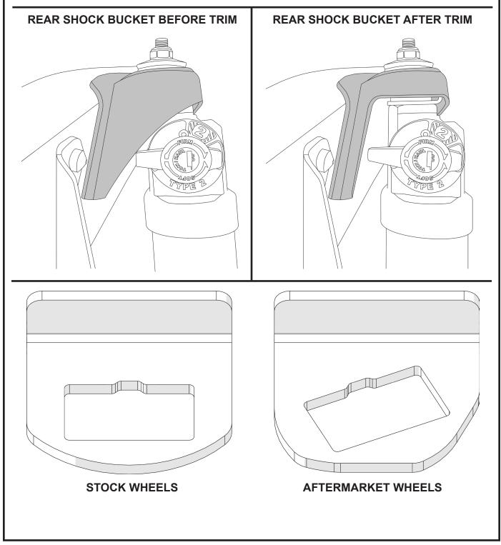
Using a tape measure make a mark 1 3/4" towards the frame and 1" down from the top of the bucket. Use a 1/2" drill bit and make a hole.
