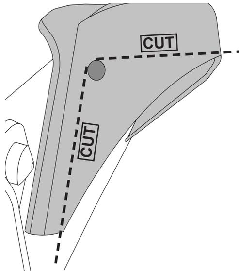
The drivers side has an extra bracket inside the shock bucket. This will also need to be cut.
