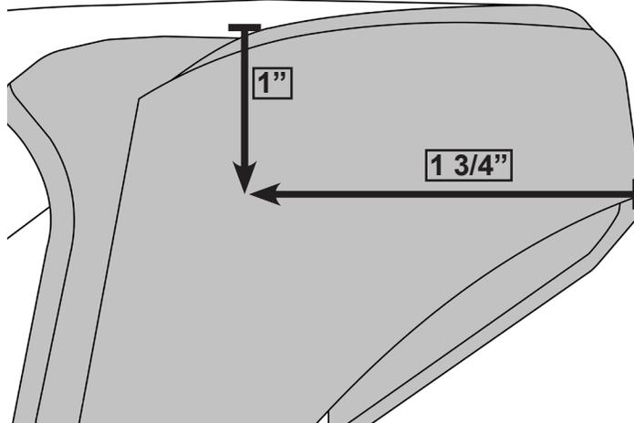
Use a Cutting Wheel to cut a straight line from the edges of the  $\frac{1}{2}$ " hole.
