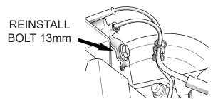
NOTE: DO NOT TIGHTEN THE CONTROL ARM BOLTS UNTIL THE JEEP IS ON THE GROUND
