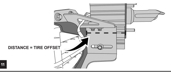
TORQUE THE SET BOLTS AND INSTALL THE SPARE TIRE AND TORQUE TO 90 FT-LBS
