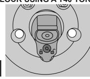
REMOVE THE TWO CAMERA HOUSING SCREWS AND TAP THE WHEEL STUDS WITH A HAMMER TO LOOSEN THE CAMERA FROM THE TIRE CARRIER
