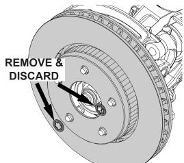
NOTE: JL MODELS USE T30 SCREWS IN PLACE OF ROTOR CLIPS
