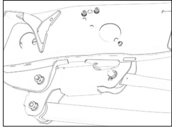
**Note:** It may be easier to align the control arms to the mount by removing the opposite side upper control arm and adjusting the axle with a hydraulic jack.
