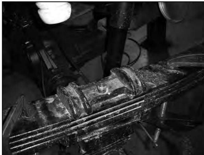
43. Remove the factory lift block. It will not be reused.
