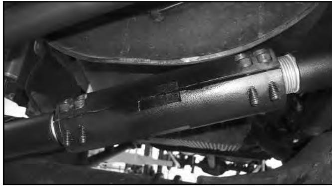
34. Adjust steering wheel to center, this will require lengthening of the drag link. Do not drive the vehicle with the steering wheel off-center for extended distances / speeds or a trip to the dealership may be required to reset the computer. Note: if there is less than 1-3/4" of thread engaged in the adjusting collar, the trackbar must be shortened to allow for adequate thread engagement of the drag link.
