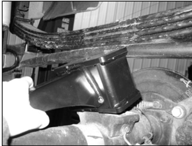
46. Repeat block installation of the driver's side. Take care not to over extend the brake lines.
