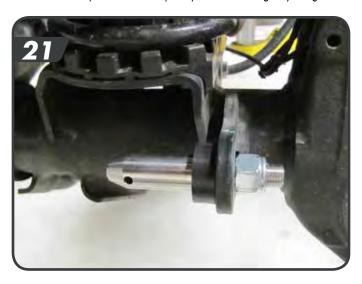
The kit comes with disconnect retention brackets to hold the links when the links are disconnected. Install the retention brackets using the provided 5/16" bolts into the factory hole in the front of the coil bucket [21]. These are designed to slightly interfere with the edge of the coil bucket to hold them in place.
