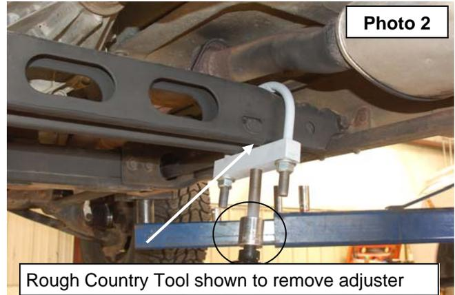
3. On the driver side, using a torsion bar removal tool, remove the stock torsion bar adjuster. Load the torsion bar using the tool and remove the bolt and threaded block. **See Photo 3.** Remove the adjuster.
