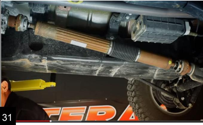
Reinstall the fuel tank in the reverse order removed. Don't forget any fuel lines, EVAP lines or electrical connections. Torque strap bolts to 30 ft-lbs.
