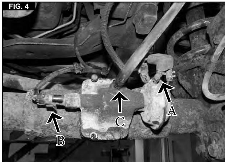
12. Remove the CAD housing and place a clean rag in the axle to eliminate the chance of debris falling in the axle. Retain wire clip from OE CAD housing. (Fig. 5-A)
