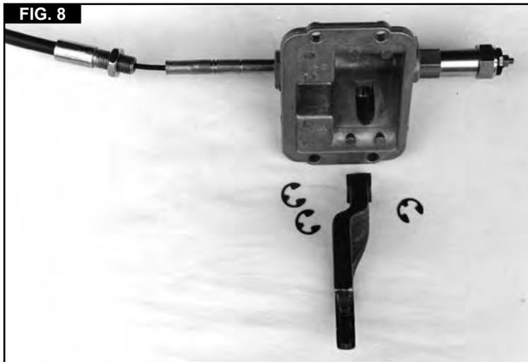
25. Press the button and pull the cable approximately 1" to the full engaged position. Check to see that the stop E-clip is resting against the housing. **Note: the CAD housing must be removed from the axle in order to adjust the fork travel. If the E-clip does not contact the housing, thread the cable out until it does.**
