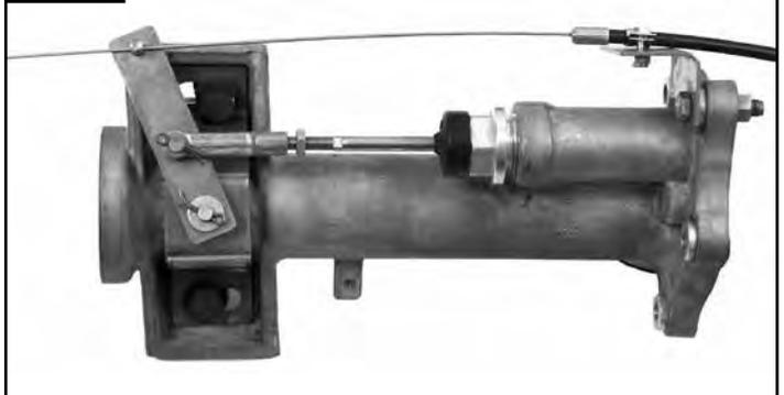
19. Push cable handle in and install the cable and cable stop in the bell crank. Place the bell crank in the unlocked position. Cut the cable off approximately 2" from the cable stop and form a loop on the end. Tighten the cable stop and align the cable bracket for smooth operation. Tighten cable bracket securely.
