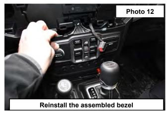
13. Reinstall the factory switch bezel removed in Step 2 making sure to properly align the tabs and popping the bezel back into place.
